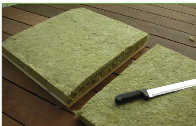
Rockwool, the growing medium of a Vertical Landscape being prepared in modules.
